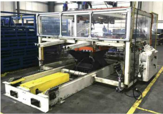
Shown here is the exit (chain conveyor) for removing two sets of stacked parts simultaneously, and extension arms used to address tayout issues.
