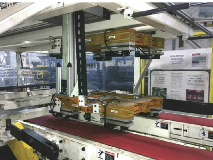
Shown here are the stacker's dual part-carrying gantries.
