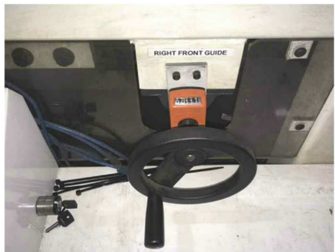
One of the five precision adjusters used for setting part-nesting stops. They help ensure precision stacking of the irregularly shaped blanks.
